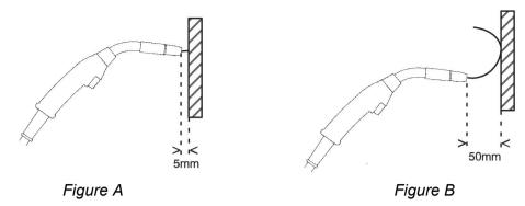
To check that the feed pressure is set correctly, you can feed out the wire against an insulated object, e.g. a piece of wood.
